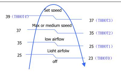
\* Residue heat sending. The indoor fan will send the residue heat at a low speed for 20 seconds. If other conditions are satisfied, when the compressor stops, the indoor system will operate at a light speed. The indoor fan will stop when the coil temperature is below the 'THHOTo'.
